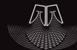
Destructive interference between conventional HF horns
