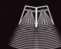
Polyhorn™ creates smoothly curved wavefront
