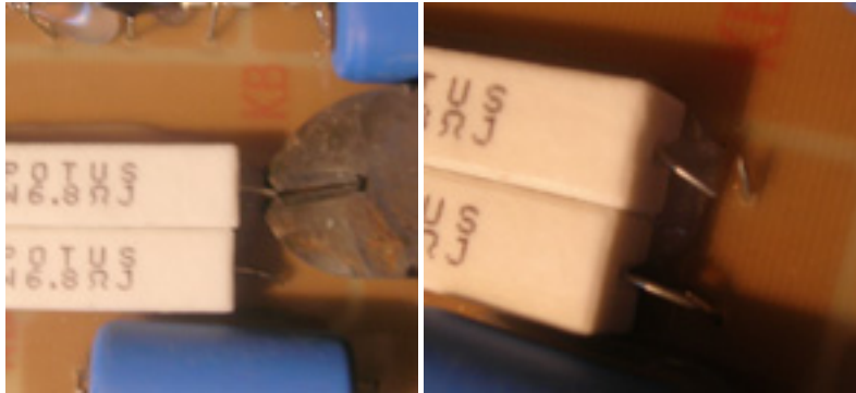
fig. 3 Snipping one of the leadouts fig. 4 Severed wire ends
